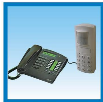
Once armed the PIR sensor detects movement in the protected area triggers the alarm and activate auto dialing to preset telephone number.
